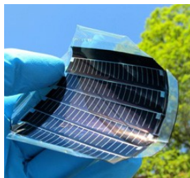
Ogniwo z tellurku kadmu CdTe
